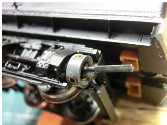
New Universal Joint Rings and bearings installed
