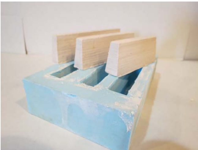
Finished cast foundations with the rubber mold
