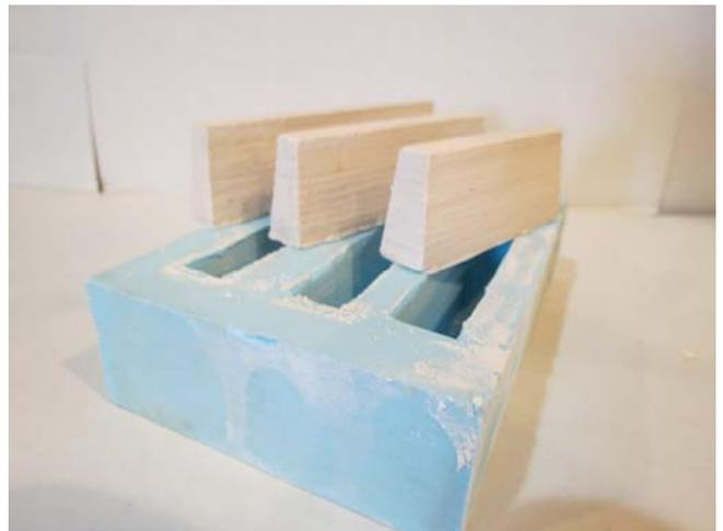
Finished cast foundations with the rubber mold
